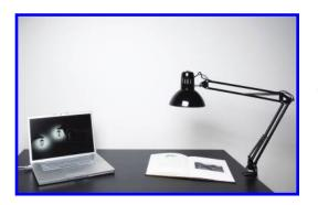
Figure 4. Our setup. The lamp acts as a normal lamp, but also hides a webcam. A standard computer processes the images captured by the webcam and adds the virtual elements. The created images are displayed on the computer screen. © 2008 Daniela Droz.
