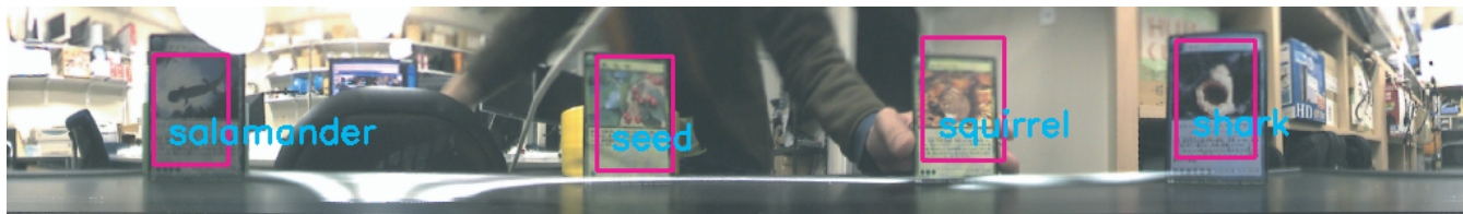
Figure 3. A result of multiple object detection. The object detection scheme is achieved in a panoramic image transformed from a omnidirectional image. In this image, four cards are shown in front of the camera, and all cards are recognized successfully. We should take note of that the annotations and the panoramic image are not displayed on the screen but shown here as just detection results.
